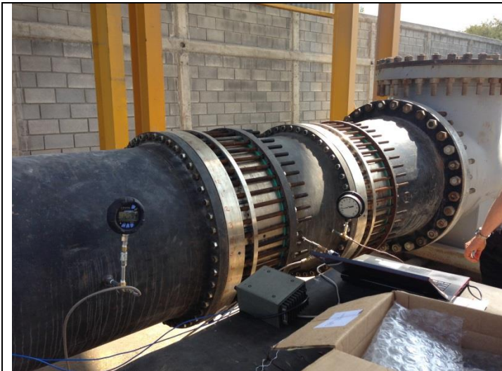
P4-1: Test Assembly: Vacuum gauge on both spools
