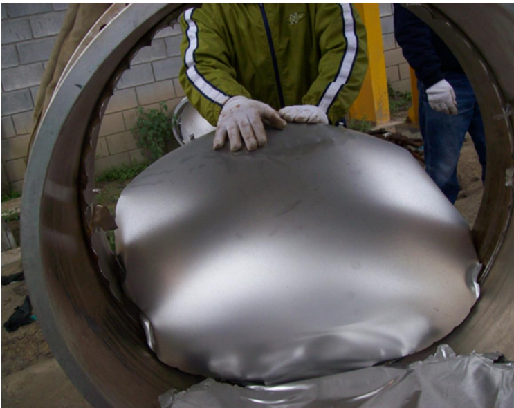
P2-5: Downstream disk (VSP-SH) is being held down in outflow direction, illustrating the minimal bending around the safety head hinge, and the reduced opening.
