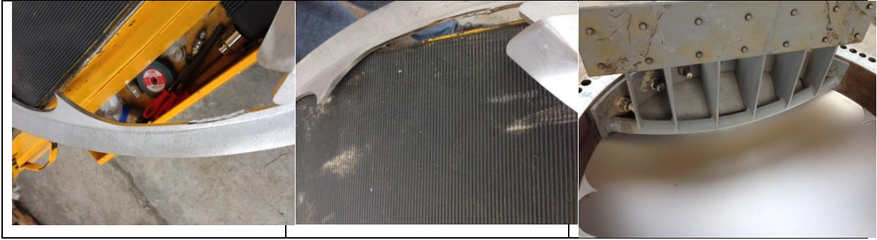
P6-2: Two half-teeth cut off on second disk low pressure JRS LP.
