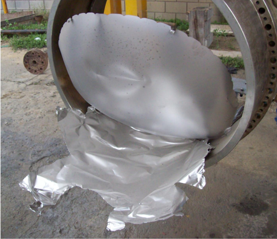
P2-4: Downstream disk (VSP-SH) with partial fragmentation of seal dome. Disk support is shown in reversed direction, as removed. Bend line is from hitting the first disk safety head hinge during reversal flow.
