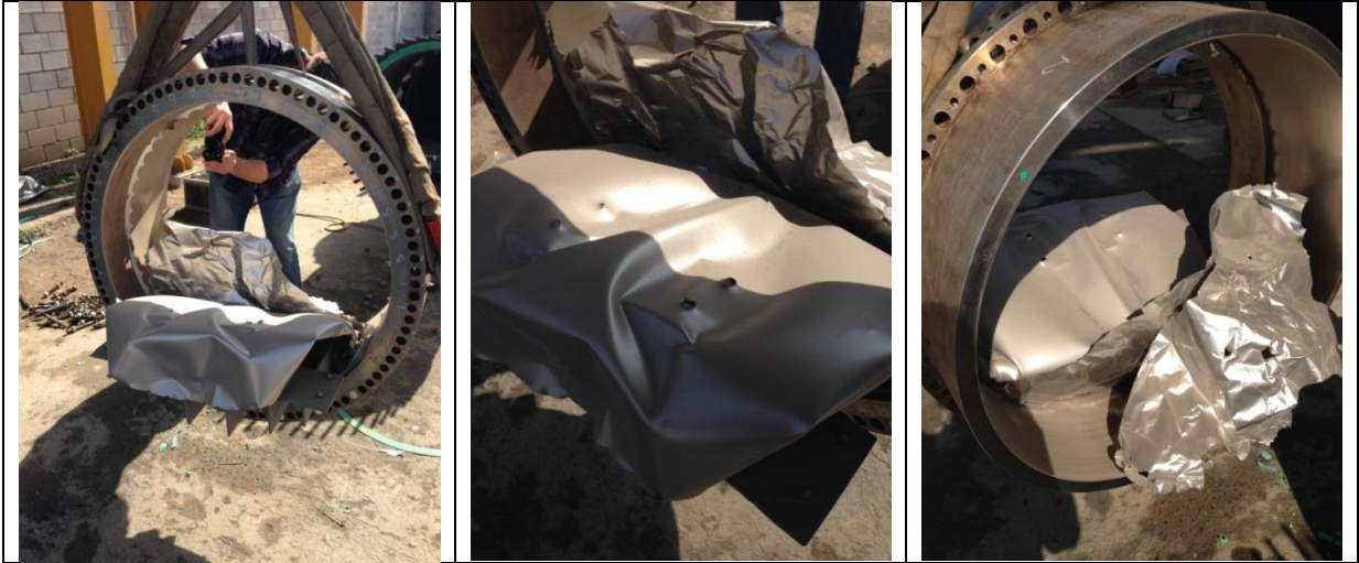
P4-7, P4-8 & P4-9: downstream low pressure VSP-SH - penetration holes and fragmentation.
