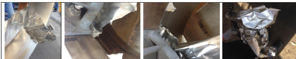
P5-12: Downstream disk (LP JRS) fragments and tear along tooth
